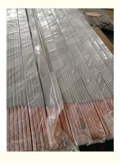
Titanium Copper CLAD BAR for Electrolysis under Strong Corrosion Conditions
