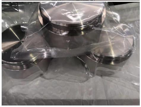
Material: titanium niobium alloy ti90nb10 Composition: Ti 90% + - 1% Nb 10% + - 1%
